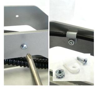
Unscrew Retaining Clip with #8-32 x ½" Screw and Nut using #2 Phillips Screwdriver
