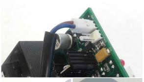
Plug Electromagnet wires into Controller port P2 (newer models) or EM1 (older models)
