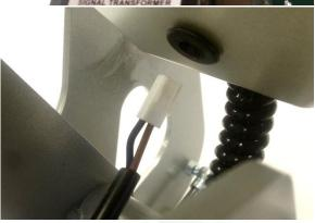
Push cable through grommet in Controller Housing to remove
