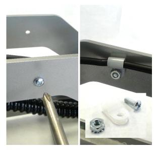
Install Retaining Clip with #8-32 x ½" Screw and Nut using #2 Phillips Screwdriver
