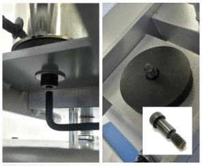
While holding  $\frac{1}{4}$ "-20 x 5/16" D x  $\frac{1}{2}$ " L" Shoulder Bolt still using 5/32" Allen Wrench, rotate old Electromagnet to unscrew
